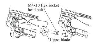
3. If the clearance is bigger than 0.25 mm, set Thin washer 5 between Blade holder and Blade.
