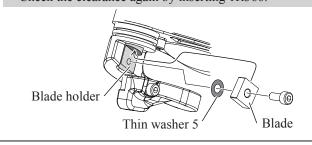
2. Make sure that the clearance of the upper and lower blades is between 0.1 - 0.25mm by inserting 1R366.
